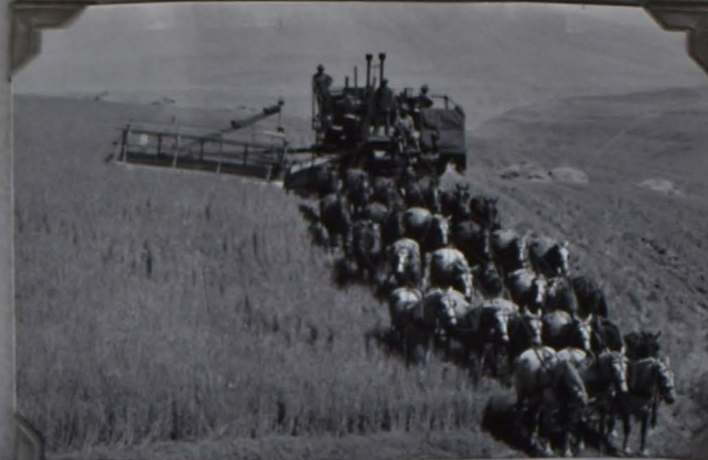
One of the early combines which was pulled by 32 horses, and operated by four men, (a driver, header tender, sack sewer, and separator tender.) When the grain was heavy a sack jig was added.
