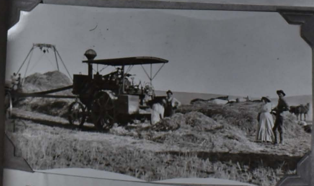
Ellis Schomp's Threshing machine in action. This machine was run by a steam powered engine.
